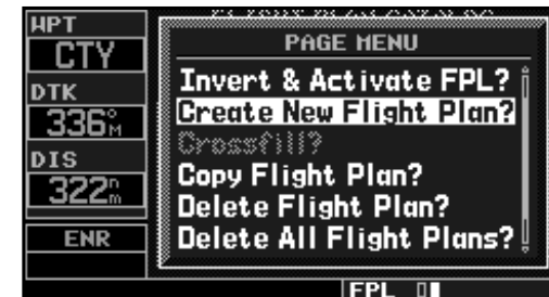
To create a new flight plan, select “Create New Flight Plan?” from the flight plan catalog options.
